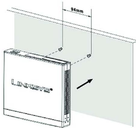
**Figure D-3: Wall-Mounting the Router**
