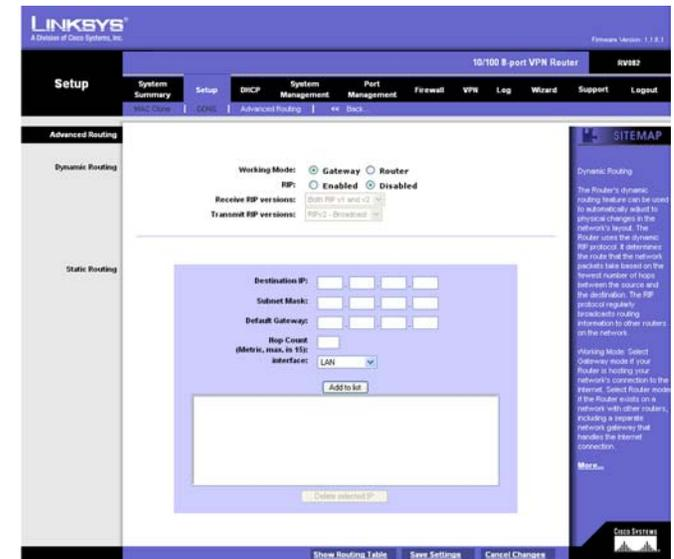
Figure 5-21: Setup Tab - Advanced Routing
