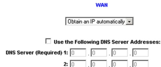
Figure 5-6: WAN Connection Type - Obtain an IP Automatically
