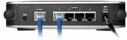
Figure 5-4: Connect the Power
