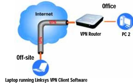
Figure 3-2: Computer to VPN Router
