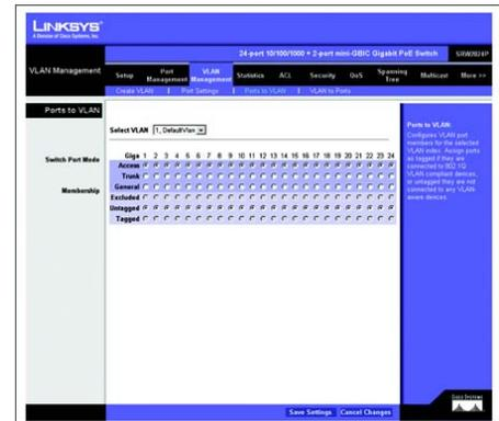
Figure 5-14: VLAN Management - Ports to VLAN
