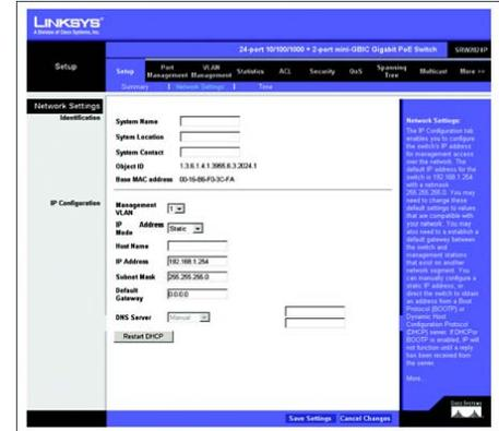
Figure 5-3: Setup - Network Settings
