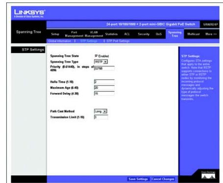
Figure 5-44: Spanning Tree - STP Settings
