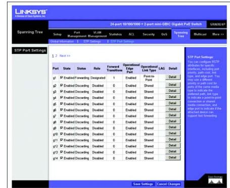
Figure 5-45: Spanning Tree - STP Port Settings
