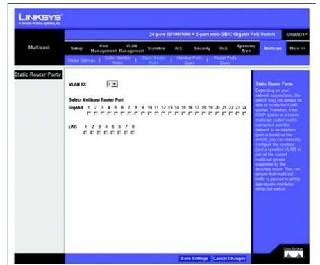
Figure 5-48: Multicast - Static Router Ports
