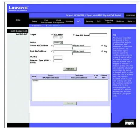
Figure 5-26: ACL - Mac Based ACL
