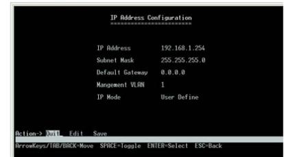
Figure 4-15: IP Address Configuration
