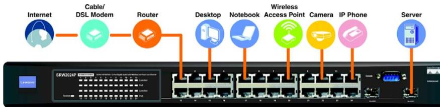
**Figure 3-1: Typical Network Configuration for the SRW2024P**
