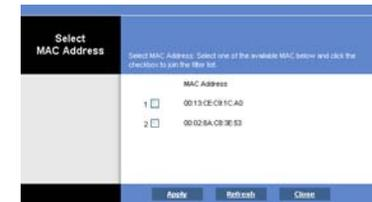
Figure 6-14: Select MAC Address from Wireless Client List
