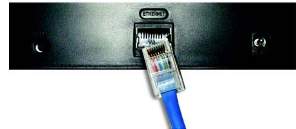
**Figure 4-1: Connect the Ethernet Cable**
