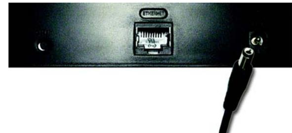
**Figure 4-2: Connect the Power**
