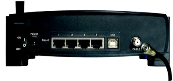
Figure 4-4: Cable Connection
