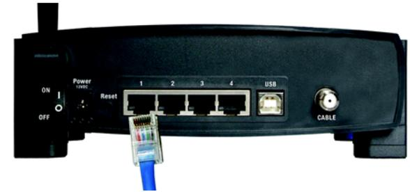
Figure 4-2: Ethernet Connection
