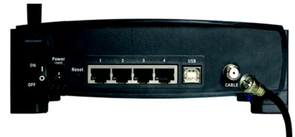
Figure 4-1: Cable Connection
