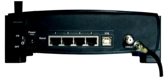
Figure 4-4: Cable Connection
