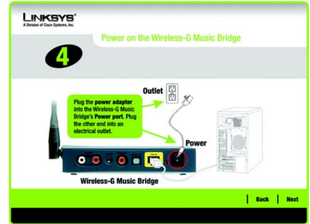
Figure 3-5: Connecting the Power
