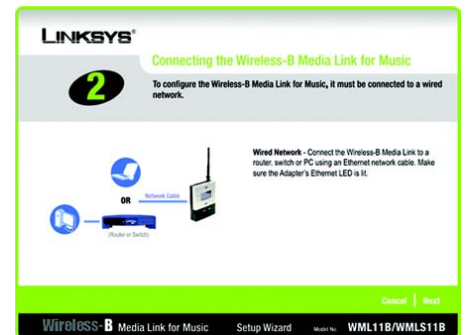
Figure 4-3: Connection for Setup Screen
