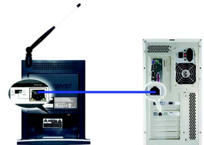
Figure 3-1: Connect the Ethernet Network Cable
