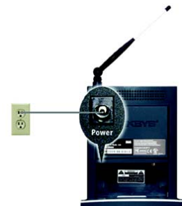
Figure 5-9: Connect the Power
