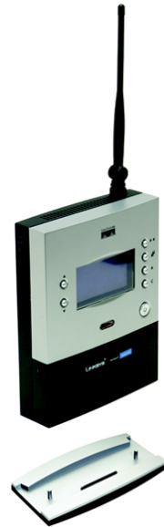
Figure 3-3: Insert the Base Plate
