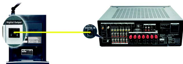
Figure 5-8: Connecting the Optical Cable to Your Stereo
