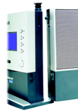
Figure 5-2: Attaching the Right Speaker
