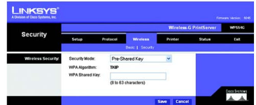
Figure 6-7: Wireless Tab - Security (Pre-Shared Key)
