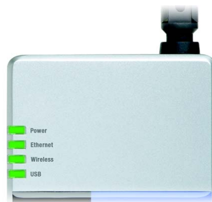
Figure 2-2: PrintServer's Front Panel
