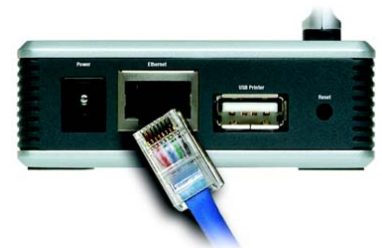
Figure 3-1: Connect to the Ethernet Port
