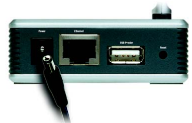
Figure 3-3: Connect to the Power Port
