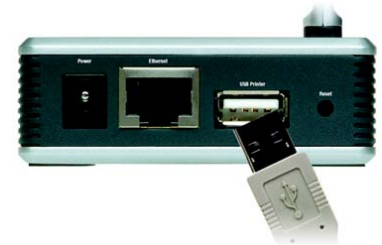
Figure 3-2: Connect to the USB Port
