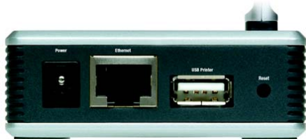
Figure 2-1: PrintServer's Bottom Panel
