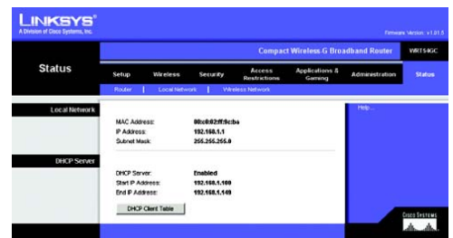
Figure 5-38: Status Tab - Router
