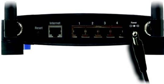
**Figure 4-8: Connecting the Power**
