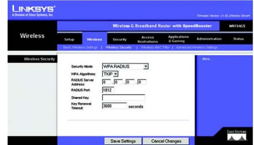
Figure 5-18: Wireless Tab - Wireless Security (WPA RADIUS)
