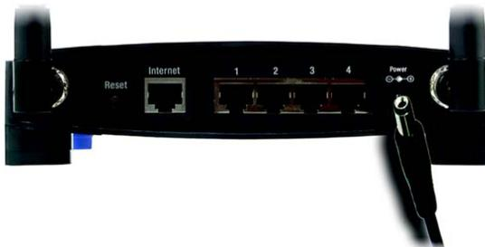
Figure 4-3: Connecting the Power
