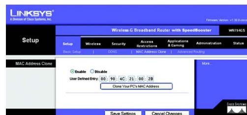
Figure 5-13: Setup Tab - MAC Address Clone
