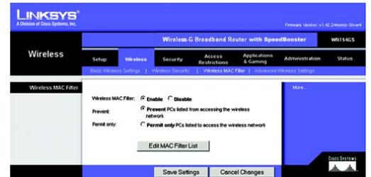
Figure 5-21: Wireless Tab - Wireless MAC Filter
