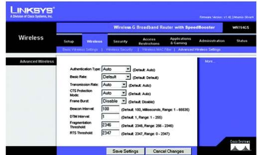
Figure 5-23: Wireless Tab - Advanced Wireless Settings
