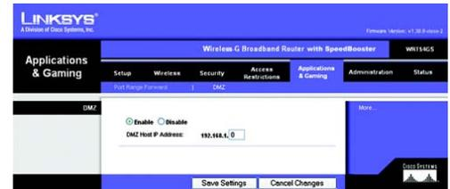
Figure 5-32: Applications and Gaming Tab - DMZ
