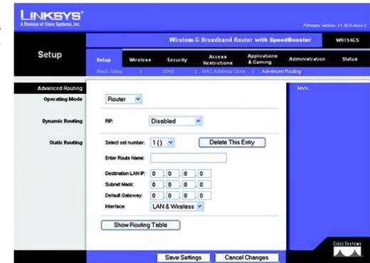
Figure 5-15: Setup Tab - Advanced Routing (Router)
