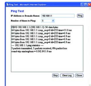
Figure 5-36: The Ping Test
