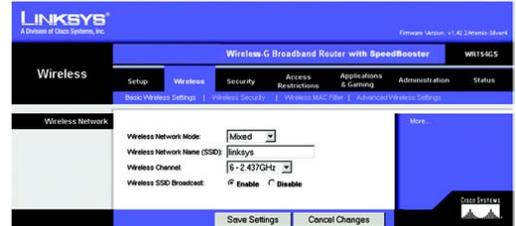
Figure 5-16: Wireless Tab - Basic Wireless Settings
