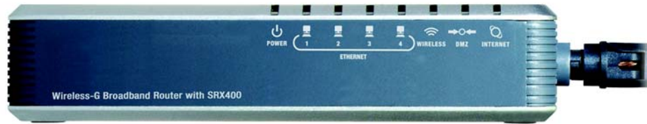
Figure 3-2: The Router's LEDs
