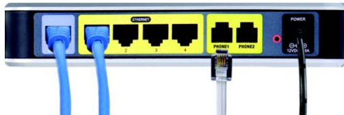
Figure 4-9: Connecting the Phone
