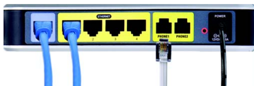
Figure 4-4: Connecting the Phone
