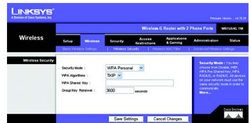
Figure 5-18: Wireless Tab - Wireless Security (WPA Personal)
