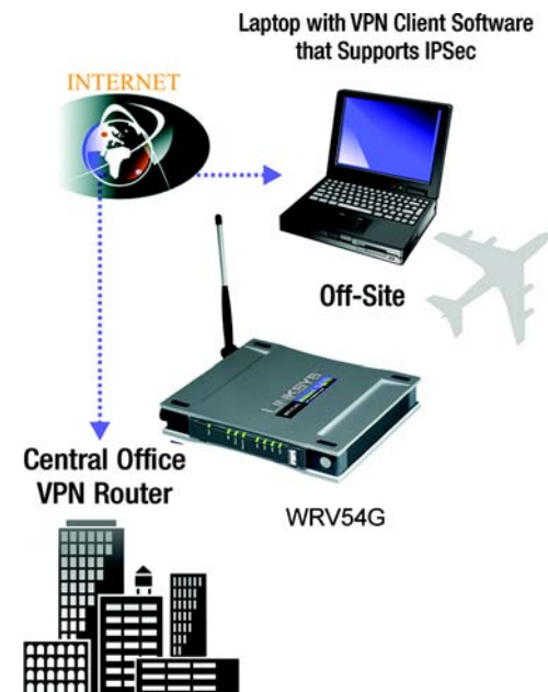
Figure 3-2: Computer to VPN Router
