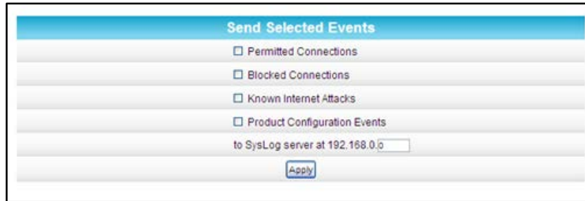
Figure 56 – Firewall Remote Log Screen
