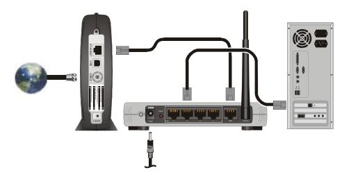
If you are connecting your PC with an Ethernet cable to the router, your PC must be installed first with an Ethernet adapter.
