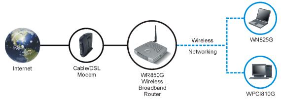
The Internet communicates with the modem which in turn communicates with the router. The router acts as the gateway to your network, sending information to whichever device asks for information, be it from requests for Internet access to file sharing to multiplayer games. The router controls the information for your network, intelligently routing the information to its required destination while at the same time protecting your network from the public domain.
