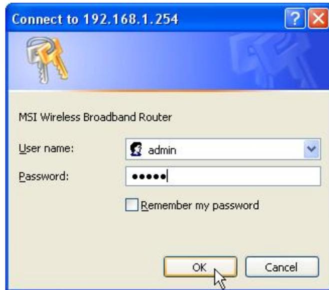
Activate your browser, and **disable the proxy** or **add the IP address of this product into the exceptions**. Then, type this product's IP address in the Location (for Netscape) or Address (for IE) field and press ENTER. For example: **http://192.168.1.254**.
