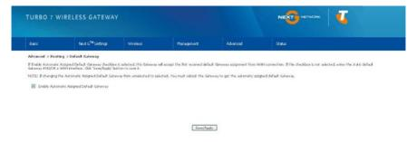
NOTE: After enabling the Automatic Assigned Default Gateway, you must re-boot the Gateway to activate the assigned default Gateway.
