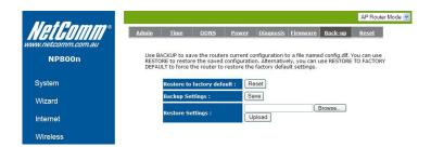
This page allows you to save the current router configurations. When you save the configurations, you also can re-load the saved configurations into the router through the Restore Settings. If extreme problems occur you can use the Restore to Factory Defaults to set all configurations to its original default settings.
