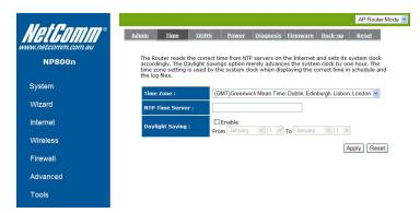
The Time Zone allows your router to reference or base its time on the settings configured here, which will affect functions such as Log entries and Firewall settings.
