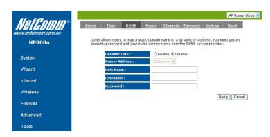
DDNS allows you to map the static domain name to a dynamic IP address. You must get an account, password and your static domain name from the DDNS service providers. This router supports DynDNS, TZO and other common DDNS service providers.
