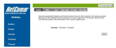
The Broadband router provides extensive firewall protection by restricting connection parameters, thus limiting the risk of hacker attacks, and defending against a wide array of common Internet attacks. However, for applications that require unrestricted access to the Internet, you can configure a specific client/server as a Demilitarized Zone (DMZ).
