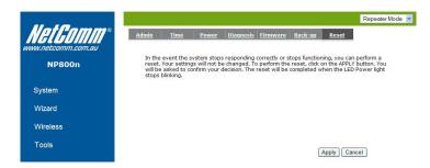
You can reset the broadband router when system stops responding correctly or stop functions.
