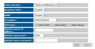
Wi-Fi Protected Access (WPA) is an advanced security standard. You can use an external RADIUS server to authenticate wireless stations and provide the session key to encrypt data during communication.
