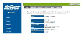
In basic setting page, you can set wireless Radio, Mode, Band, SSID, and Channel.
