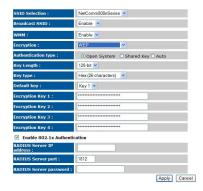
When you select 64-bit or 128-bit WEP key, you have to enter WEP keys to encrypt data. You can generate the key by yourself and enter it. You can enter four WEP keys and select one of them as a default key. Then the router can receive any packets encrypted by one of the four keys.
