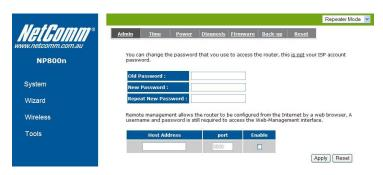
You can change the password required to log into the broadband router's system web-based management. By default, the password is: admin. Passwords can contain 0 to 12 alphanumeric characters, and are case sensitive.
