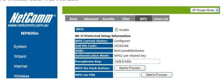
WPS: Check the box to enable WPS function and uncheck it to disable the WPS function.
