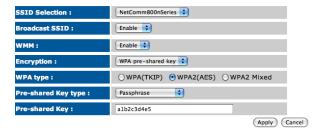
Wi-Fi Protected Access (WPA) is an advanced security standard. You can use a pre-shared key to authenticate wireless stations and encrypt data during communication. It uses TKIP or CCMP (AES) to change the encryption key frequently. So the encryption key is not easy to be cracked by hackers. This is the best security available.
