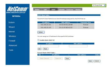
View the current LAN clients which are assigned with an IP Address by the DHCP-server. This page shows all DHCP clients (LAN PCs) currently connected to your network. The table shows the assigned IP address, MAC address and expiration time for each DHCP leased client. Use the <Refresh> button to update the available information.
