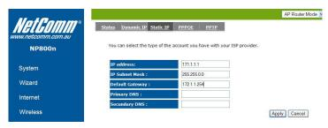
If your ISP Provider has assigned a fixed IP address, enter the assigned IP address, Subnet mask, Default Gateway IP address, and Primary DNS of your ISP provider.
