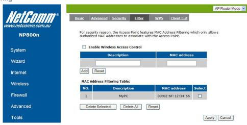
This wireless router supports MAC Address Control, which prevents unauthorized clients from accessing your wireless network.
