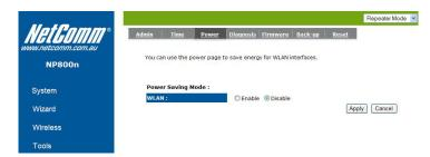
Saving power in WLAN mode can be enabled / disabled in this page.
