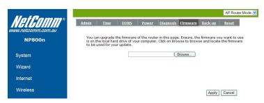
This page allows you to upgrade the router's firmware. To upgrade the firmware of your Broadband router, you need to download the firmware file to your local hard disk, and enter that file name and path in the appropriate field on this page. You can also use the Browse button to find the firmware file on your PC.
