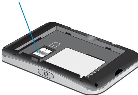
4. Ensure that the micro SIM card is seated securely.
