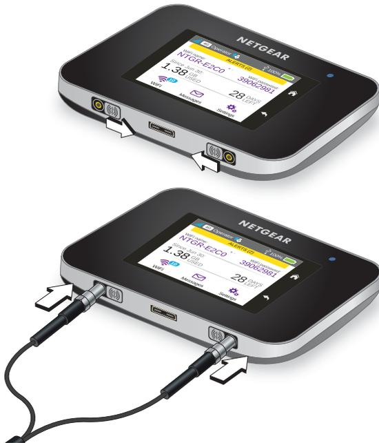
Figure 3. External antennas with TS-9 connectors
