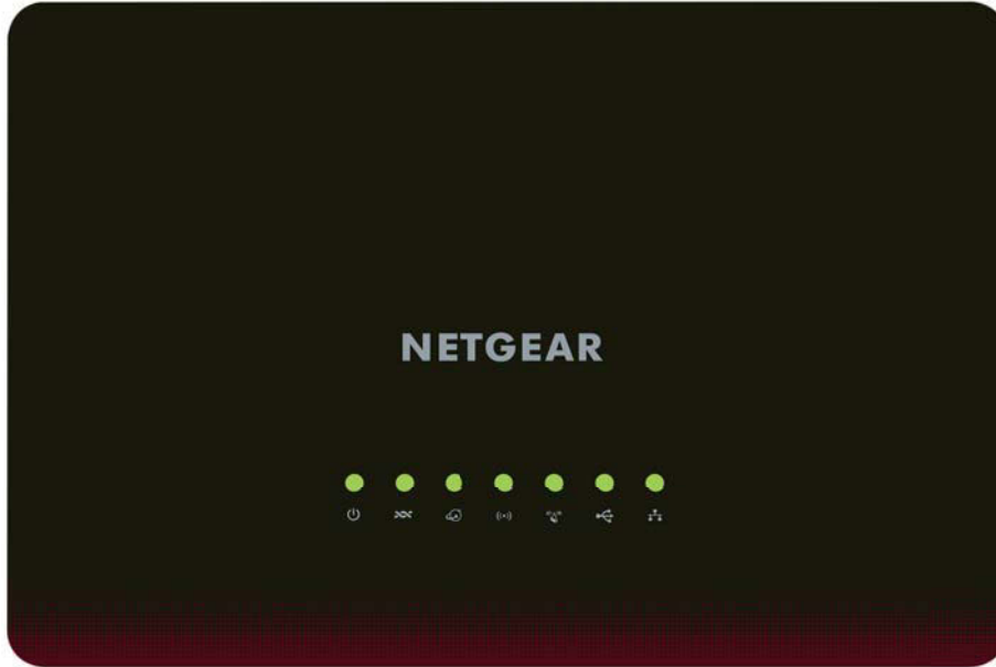
Figure 2. Modem router top panel with LEDs
