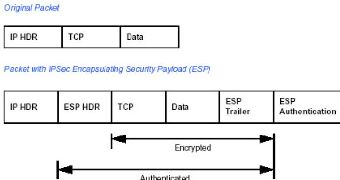
**Figure C-1: Original packet and packet with IPSec Encapsulated Security Payload**
