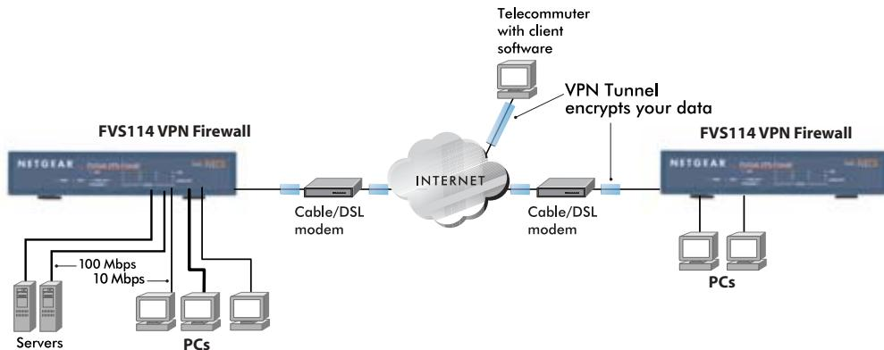
**Figure 6-1: Secure access through FVS114 VPN firewalls**
