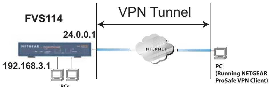
**Figure 5-3: Client-to-gateway VPN tunnel**
