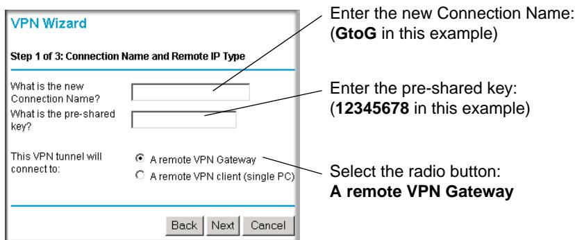
**Figure 5-24: Connection Name and Remote IP Type**
