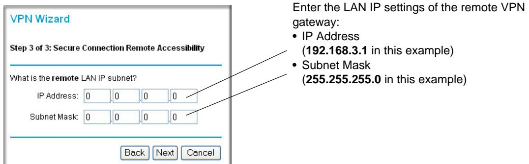
**Figure 5-26: Secure Connection Remote Accessibility**
