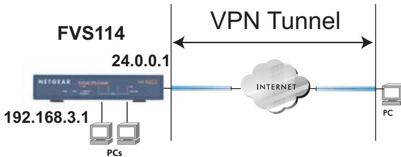
**Figure 5-1: Client-to-gateway VPN tunnel**
