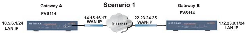
**Figure 6-6: LAN to LAN VPN access from an FVS114 to an FVS114**
