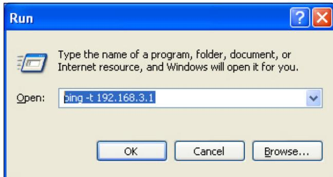
**Figure 5-34:** Running a Ping test to the LAN from the PC
