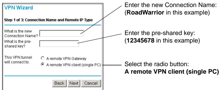
**Figure 5-5: Connection Name and Remote IP Type**
