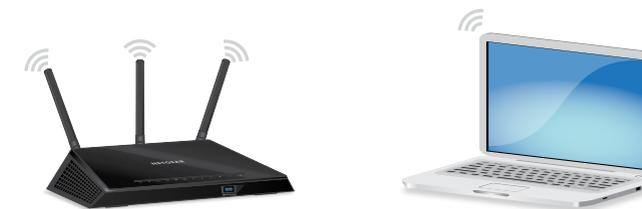
Make sure that the router's WiFi LED (
