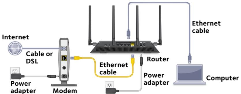
You can use an Ethernet cable to connect a computer to the router or you can use WiFi to connect a computer or WiFi device to the router:
