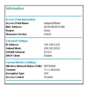
Figure 4-1: Wireless Access Point Status screen
