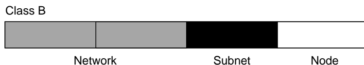
Figure 7-2: Example of Subnetting a Class B Address
