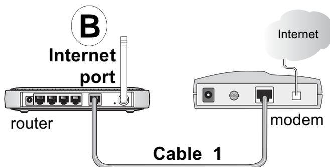
**Figure 3-2: Connect the wireless router to the modem**
