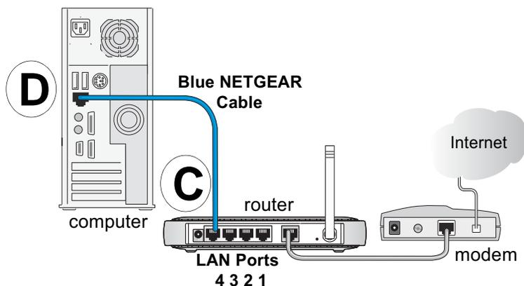
**Figure 3-3: Connect the computers on your network to the router**
