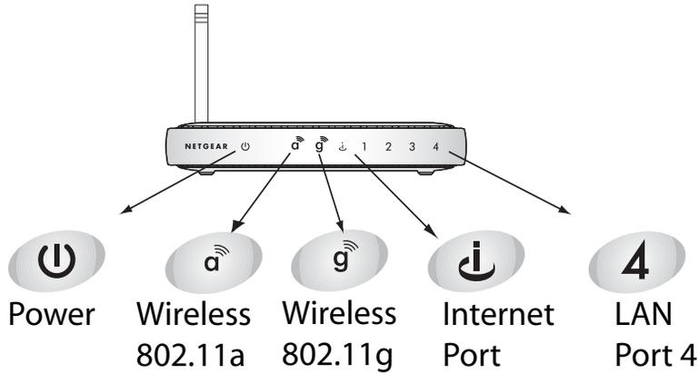
**Figure 2-1: WGU624 Front Panel**
