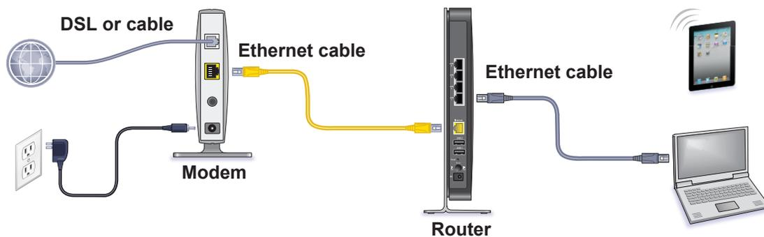
Figure 4. Router cabling
