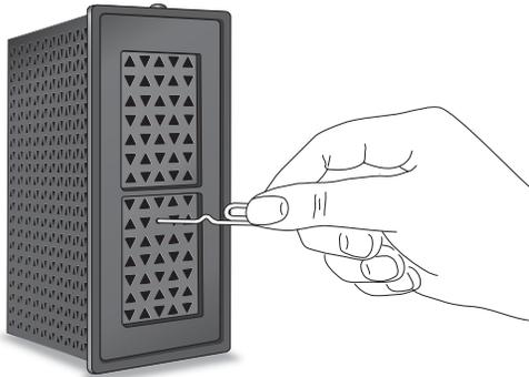
The router resets and returns to the factory configuration settings shown in the following table.
