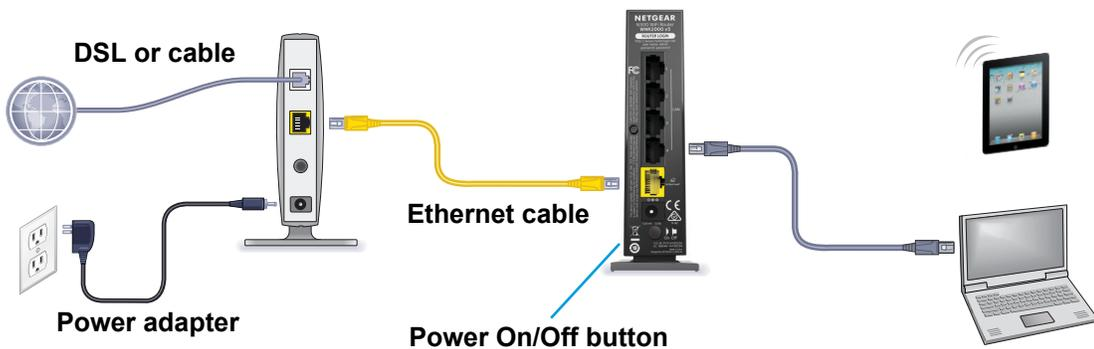
2. Press the **Power On/Off** button on the rear panel of the router.
