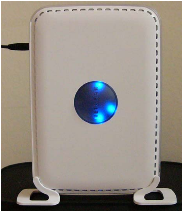
Figure 4-1: Vertical orientation required on metallic surfaces
