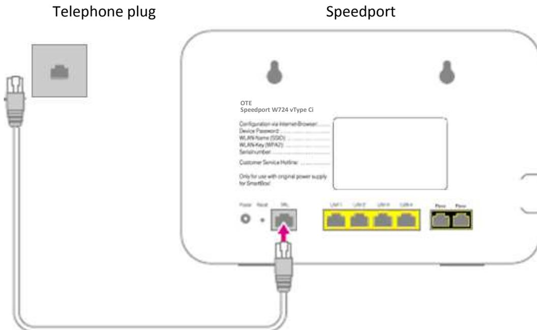
**Notice:** If you use a broadband connection with splitter, connect the DSL plug of the splitter and the DSL plug of your Speedport with the DSL cable for the connection with splitter (RJ11/RJ11, grey plug).
