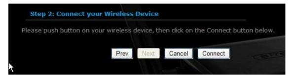
Press the **WPS** button on the device (which is located on the left side of the front panel) and then click on the **Next** button.
