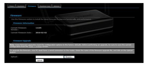
Ensure that you have downloaded the appropriate firmware from the vendor's website. Connect the device to your PC using an Ethernet cable, as the firmware cannot be upgraded using the wireless interface.
