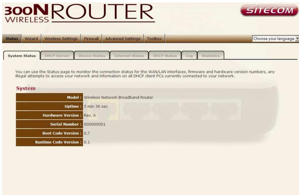
The System status section allows you to monitor the current status of your router the UP time, hardware information, serial number as well as firmware version information is displayed here.
