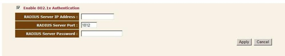
The screenshot shows the 'Enable 802.1x Authentication' section of the security configuration page. The checkbox for 'Enable 802.1x Authentication' is checked. Below it, there are three input fields: 'RADIUS Server IP Address' (empty), 'RADIUS Server Port' (set to 1812), and 'RADIUS Server Password' (empty). At the bottom right, there are 'Apply' and 'Cancel' buttons.
