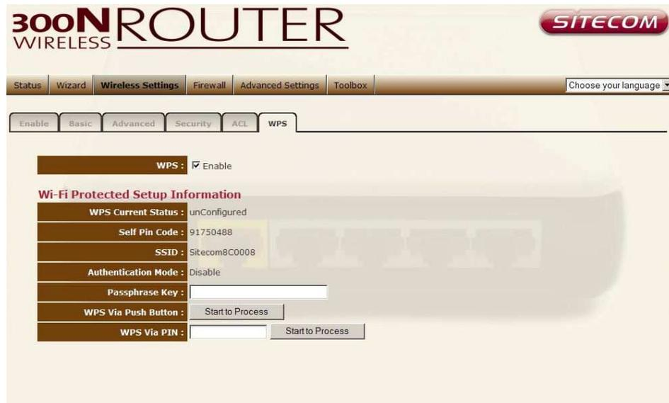
The screenshot shows the web configuration interface for a 300N WIRELESS ROUTER. The interface includes a navigation menu with options like Status, Wizard, Wireless Settings, Firewall, Advanced Settings, and Toolbox. The 'Wireless Settings' section is active, and the 'WPS' tab is selected. The WPS settings are as follows:
