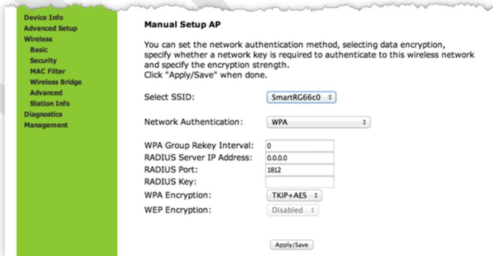
The screenshot shows the 'Manual Setup AP' configuration page. On the left is a navigation menu with options: Device Info, Advanced Setup, Wireless, Basic, Security, MAC Filter, Wireless Bridge, Advanced, Station Info, Diagnostics, and Management. The main content area is titled 'Manual Setup AP' and includes the following fields:
