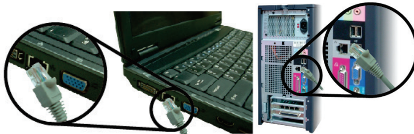
Figure 4. Connecting the Gateway to a Laptop or Desktop Computer
