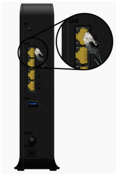
Figure 3. Connecting to a LAN Port on the Gateway Rear Panel
