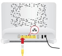
2 Connect the other end of the Ethernet cable to your network device.
