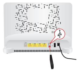
By using a USB hub, you can connect up to five USB mass storage devices to the TG589vn v3.
