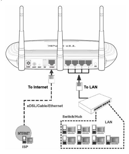
Figure 2-1 Hardware Installation
