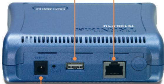
3. Connect the **AC Power Adapter** to the Print Server and then to a power outlet.
