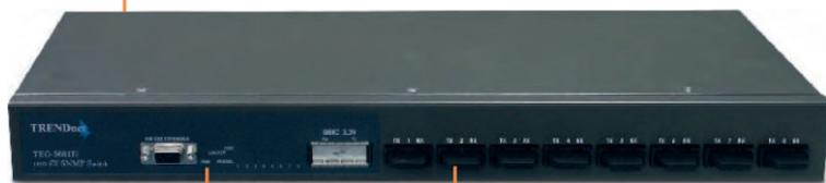
2. Connect the fiber cable to the front of the switch and your Network.
