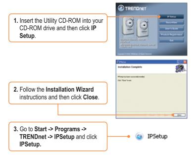
Note: By default, the IP setting on the TV-IP110/TV-IP110W is set to DHCP. Please skip to step 8. If you want to give the TV-IP110/TV-IP110W static IP address, continue on to step 4.
