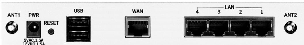
**Figure 1: ZoneAlarm Z100G Router Rear Panel**
