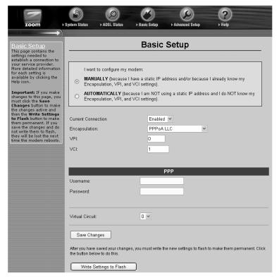
Use this Web page to configure the modem so it can connect with your Internet service provider. You can configure the X5 manually or you can have the modem automatically configure itself.
