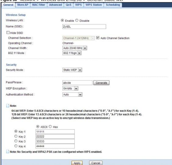
Figure 58 Network > Wireless LAN 2.4G/5G > General: Static WEP
