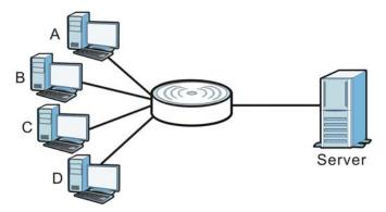
In the multicast example above, systems A and D comprise one multicast group. In multicasting, the server only needs to send one data stream and this is delivered to systems A and D.
