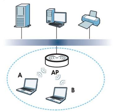
The wireless network is the part in the blue circle. In this wireless network, devices **A** and **B** are called wireless clients. The wireless clients use the access point (AP) to interact with other devices (such as the printer) or with the Internet. Your NBG6716 is the AP.
