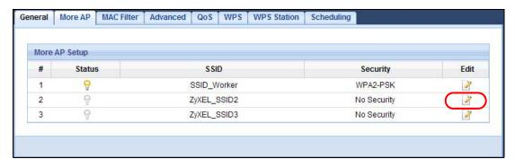
11 Configure the screen as follows. You do not enable Intra-BSS Traffic for SSID\_VoIP. Click Apply.
