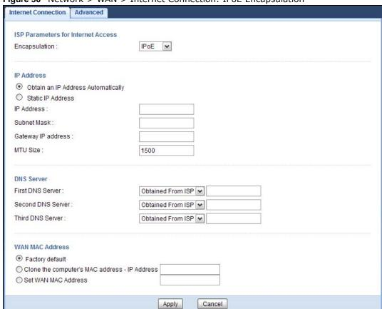
Figure 50 Network > WAN > Internet Connection: IPoE Encapsulation
