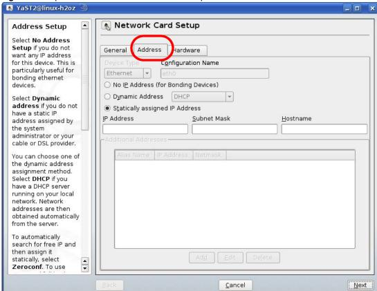
Figure 145 openSUSE 10.3: Network Card Setup
