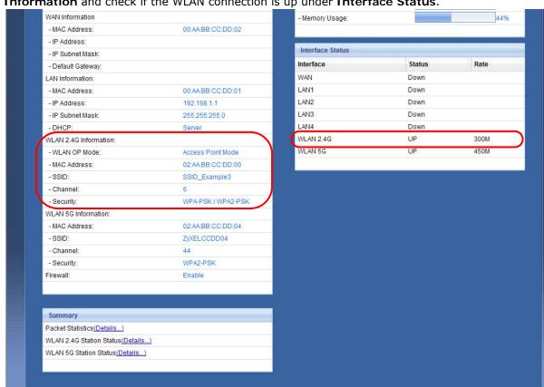
Open the **Status** screen. Verify your wireless and wireless security settings under **Device**Information and check if the WLAN connection is up under Interface Status.
