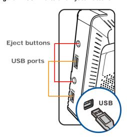
Note: For the USB function, it is strongly recommended to use version 2.0 or lower USB storage devices (such as memory sticks, USB hard drives) and/or USB devices. Other USB products are not guaranteed to function properly with the NBG6716.
