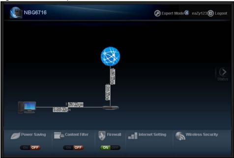
You can view the upstream and downstream transmission speed between the NBG6716 and the Internet and/or between the NBG6716 and the connected device(s) (represented by icons indicating the kind of network device), including those connecting wirelessly.
