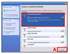
You are prompted to enter a password. Enter the encryption key (WPA-PSK) found in the back panel of the P-2812HNU(L)-Fx Series and click Connect.
