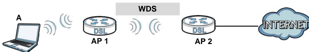
Figure 50 WDS Link Example
