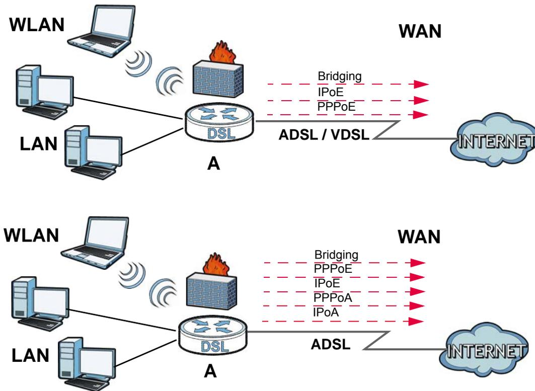
You can also configure IP filtering on the Device for secure Internet access. When the IP filter is on, all incoming traffic from the Internet to your network is blocked by default unless it is initiated from
