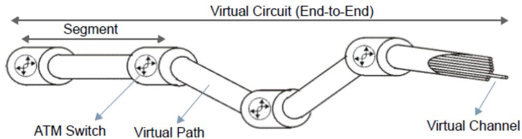
Think of a virtual path as a cable that contains a bundle of wires. The cable connects two points and wires within the cable provide individual circuits between the two points. In an ATM cell header, a VPI (Virtual Path Identifier) identifies a link formed by a virtual path; a VCI (Virtual Channel Identifier) identifies a channel within a virtual path. A series of virtual paths make up a virtual circuit.
