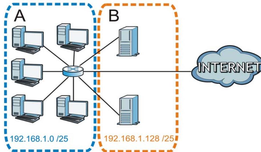
In a 25-bit subnet the host ID has 7 bits, so each sub-network has a maximum of  $2^7 - 2$  or 126 possible hosts (a host ID of all zeroes is the subnet's address itself, all ones is the subnet's broadcast address).
