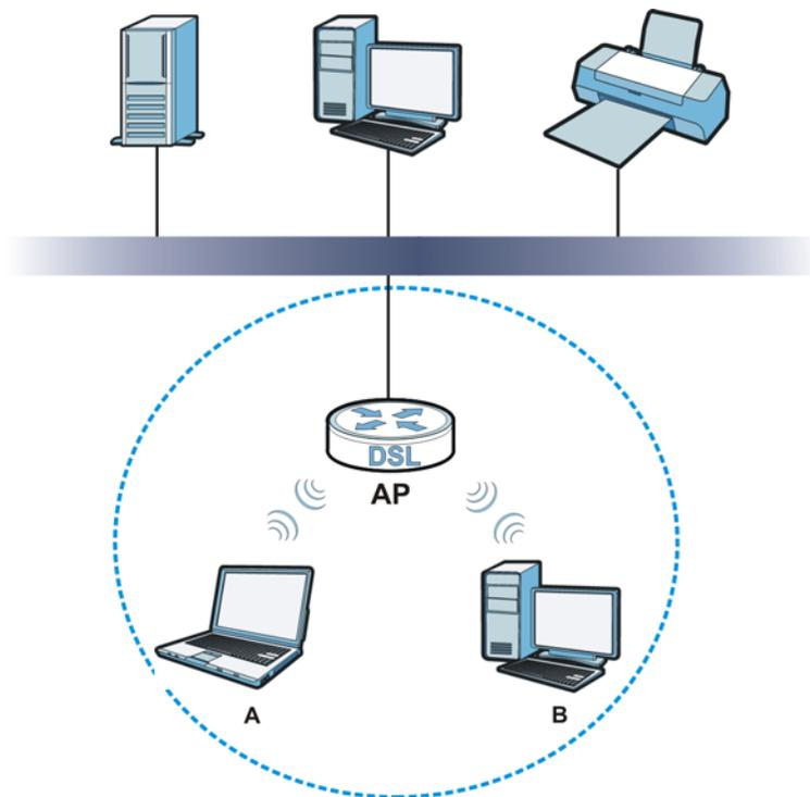
The wireless network is the part in the blue circle. In this wireless network, devices **A** and **B** use the access point (**AP**) to interact with the other devices (such as the printer) or with the Internet. Your Device is the AP.
