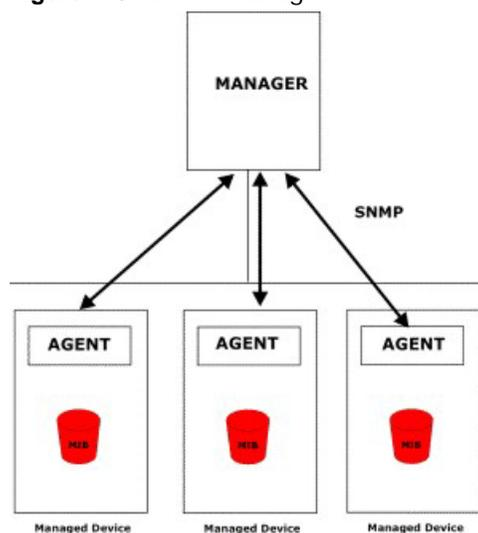
An SNMP managed network consists of two main types of component: agents and a manager.
