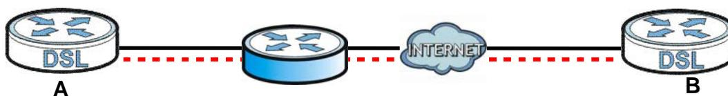
Normally you cannot set up an IKE SA with a NAT router between the two IPSec routers because the NAT router changes the header of the IPSec packet. NAT traversal solves the problem by adding a UDP port 500 header to the IPSec packet. The NAT router forwards the IPSec packet with the UDP port 500 header unchanged. In the above figure, when IPSec router **A** tries to establish an IKE SA, IPSec router **B** checks the UDP port 500 header, and IPSec routers **A** and **B** build the IKE SA.
